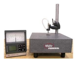
Surface plates provide a stable reference surface on a large scale, making a great many gaging setups possible on a single, simple piece of equipment. When a gaging application does not warrant the purchase of a special-purpose fixture gage, a surface plate itself can also be a gage.
