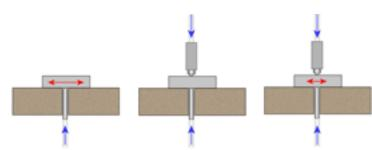
A hole is bored in the plate, and a gage head or air jet installed to inspect flush surfaces for flatness without the use of a height stand. A second gage head in a height stand can be positioned directly above the one embedded in the surface plate, permitting independent measurements of flatness, thickness, and parallelism.
