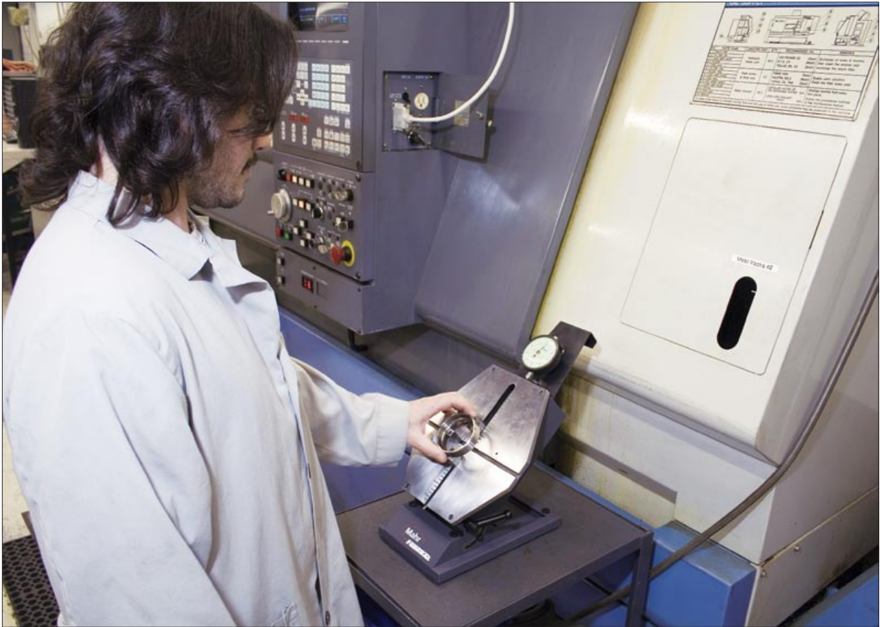
An operator uses a T-plate bench-mounted comparator gage to check an ID. Source: Mahr
