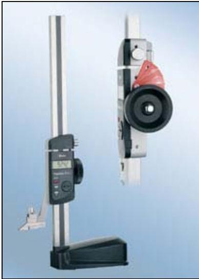
The digital height gage allows for direct reading of part height or scribing as part of a layout operation. A locking mechanism is released for fast positioning of the scriber while a fine adjust allows for precise position.
