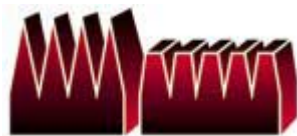
Fig. 2 - The Rk family of parameters describes multifunctional surfaces, such as cylinder walls. On the illustration, the section on the left shows the surface after initial rough cutting. Plateau honing knocks off the tops of the peaks, as shown on the right. In operation, this surface has sufficient area to promote piston compression, with enough pockets to hold lubricating oil.
