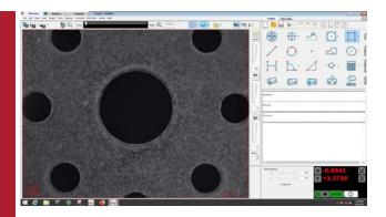
Transform the traditional optical comparator into a fully automatic inspection system with optional VidiProbe and SNAP-X $^{\text{TM}}$  software. The video camera is internally mounted to enable simultaneous measurements using both the analog comparator screen and the digital video with SNAP-X.
