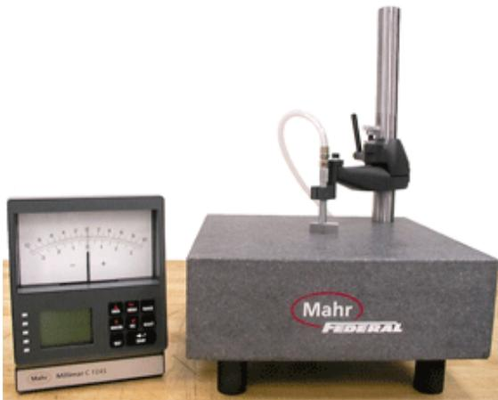
Surface plates provide a stable reference surface on a large scale, making a great many gaging setups possible on a single, simple piece of equipment. When a gaging application does not warrant the purchase of a special-purpose fixture gage, a surface plate itself can also be a gage.
