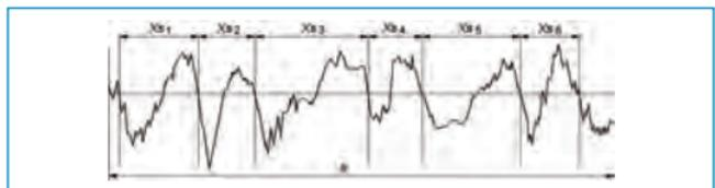
**Fig. 9:** The material ratio curve of the profile plots the material portion  $Rmr(c)$  of the profile as a function of the section height  $c$  (Abbott-Firestone curve)
