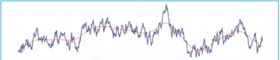
Fig. 1: Primary profile after  $\lambda_s$  low-pass filtering
