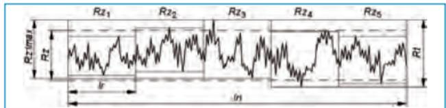
The average groove width is the mean value of the width  $i$  of the profile elements
