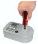
Some other applications require more than just the peak. Certain tests call for the torque profile to be recorded and used to further analyze the behavior of the sample. Using the example of the bottle cap once more, analyzing the torque profile may highlight problem areas in the thread or other aspects of the cap. Materials testing of metals and plastics also often requires such testing, as well as the testing of components such as latches, bearings, connectors and springs.
